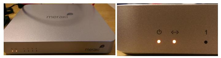
To reboot the router unplug the power lead from the back and plug back in after 10 seconds.
